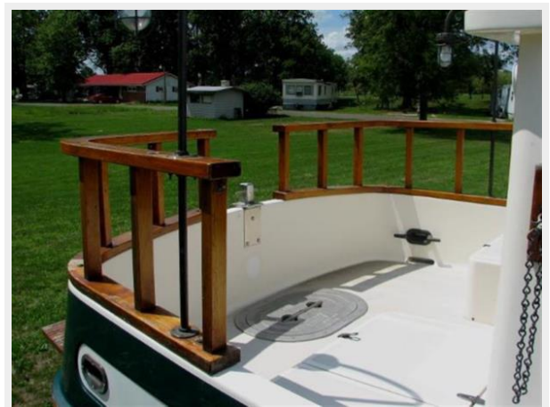
Aft Deck Railing
