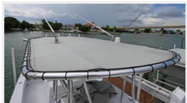
T-Top W/VHF, Radio, & GPS Antennas
