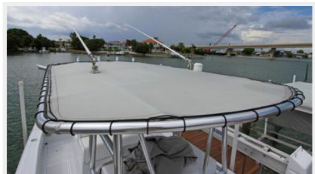
T-Top W/VHF, Radio, & GPS Antennas
