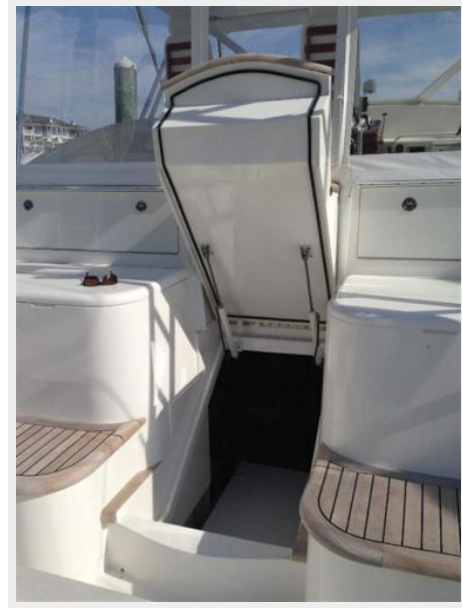
Engine Room Access
