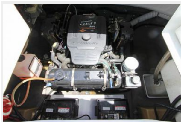
MerCruiser 300 HP 350 MPI Freshwater Cooled Engine
