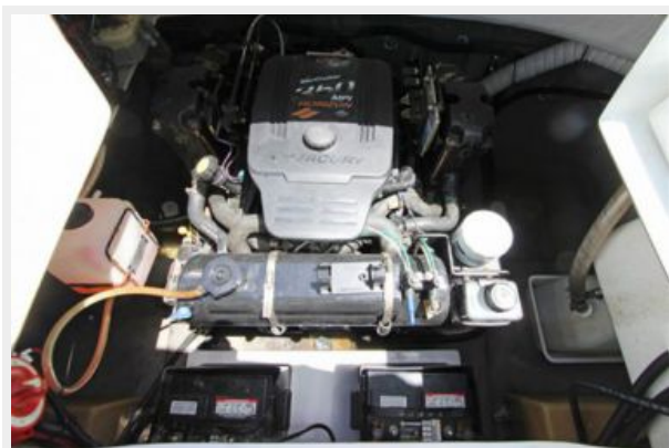
MerCruiser 300 HP 350 MPI Freshwater Cooled Engine
