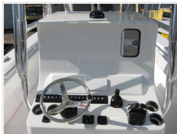
Helm w/ Yamaha Joystick control
