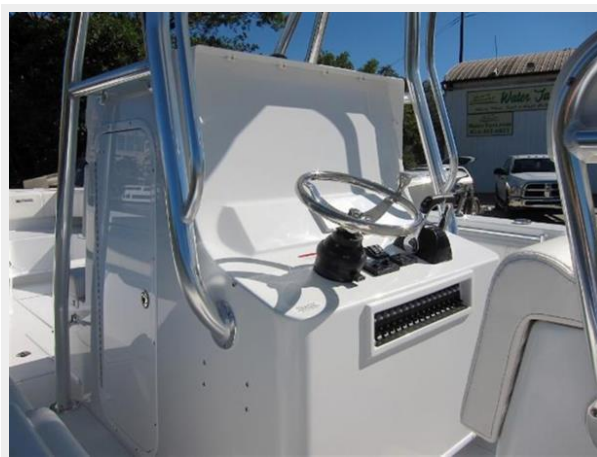
Console w/ side entry door
