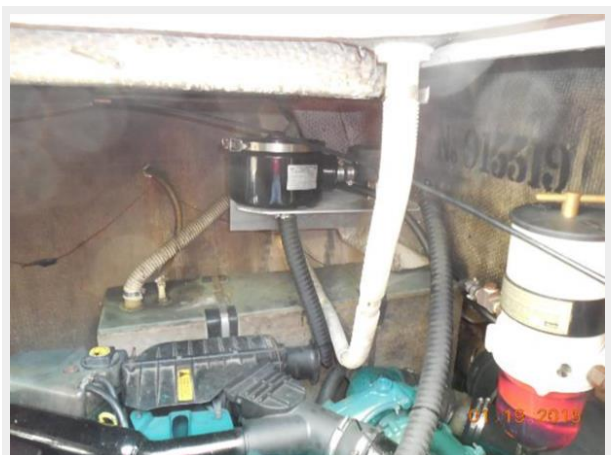
34' Luhrs Open, racor filters
